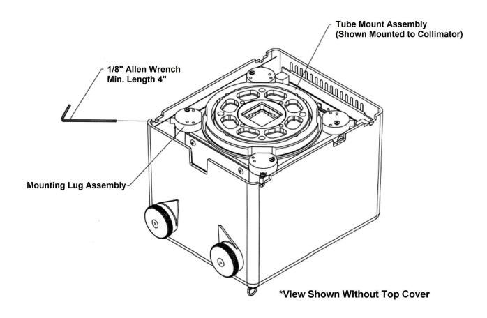
Figure 4 - Collimator Tube Mount Assembly Installation
