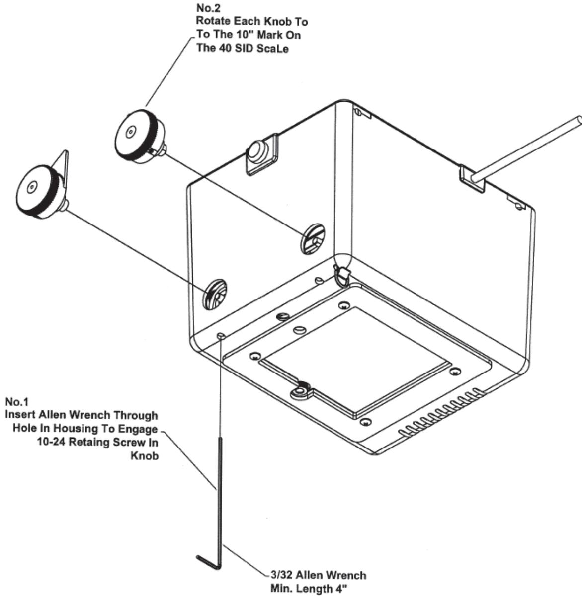
Figure 5 - Control Knob Removal
