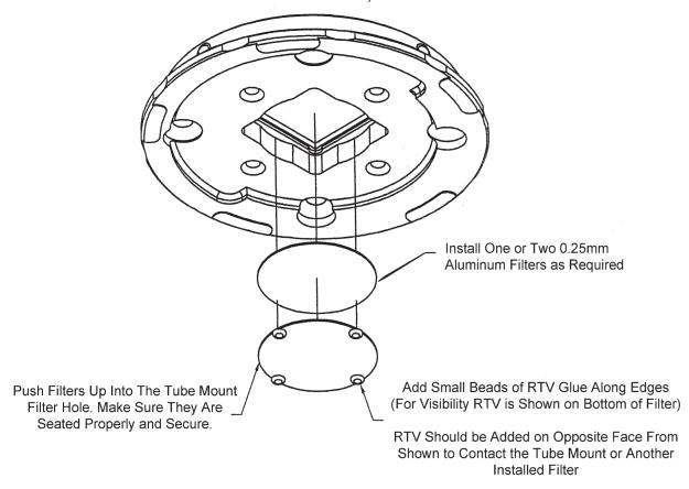
Figure 3 - Filtration Installation
